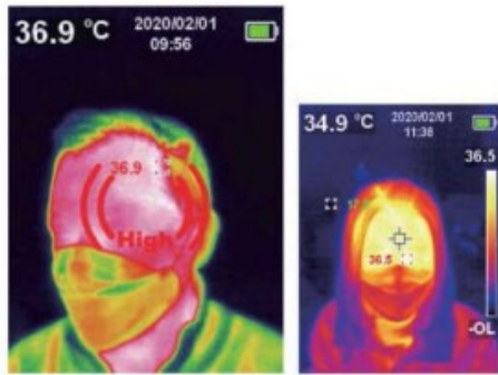
HI/LO Temperature Alarm: Central point temperature measurement, high/low temperature auto tracking and real-time temperature display.
